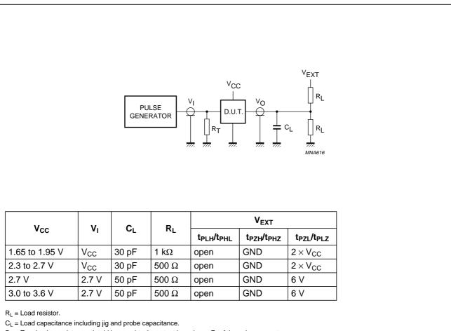
$R_T$  = Termination resistance should be equal to the output impedance  $Z_0$  of the pulse generator.
