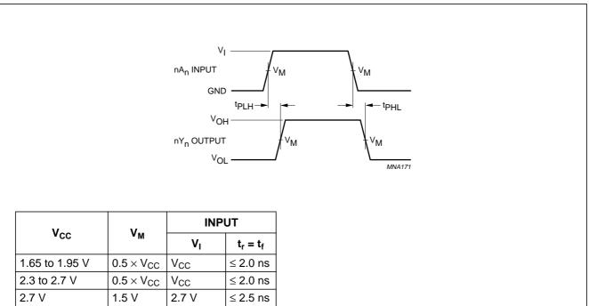
Fig.5 Input  $nA_n$  to output  $nY_n$  propagation delay times.
